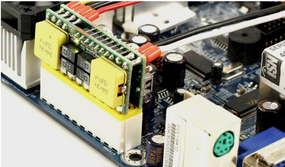
2) Connect a 12 VDC power adapter (or any 12V source) to the DC-to-DC connector, center pin / white wire is positive (+).
